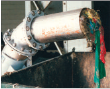
Rags are dewatered along with the screenings. There are no sharp edges to snag rags and jam equipment.
