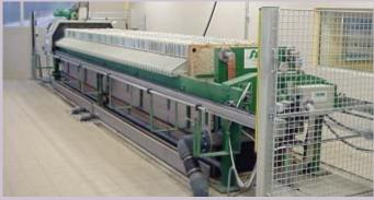
**Deselec™** is an advanced electro-dewatering system combining the benefits of dewatering and partial drying to minimize disposal costs. Electro-dewatering involves the use of an electric field during mechanical dewatering.
