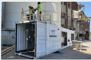
**MOBILE LIME SLURRY – PRODUCTION**Fully Autonomous Slaking Solution
